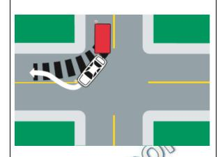
Turning right when towing a trailer—note path of the vehicle and trailer wheels. 右转,注意前车和拖挂车的行车轨迹。
