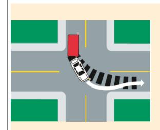
Turning left when towing a trailer - note path of the vehicle and trailer wheels.
